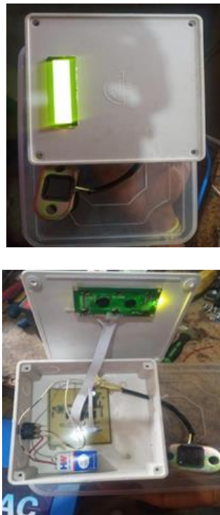
Figure 10: The proposed digital fuel level indicator (a) Internal connection (b) external features. The problems encountered during the development of the system are highlighted below:
