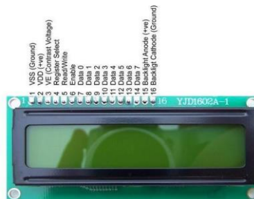
Figure 3: Pin Connection of the LCD
