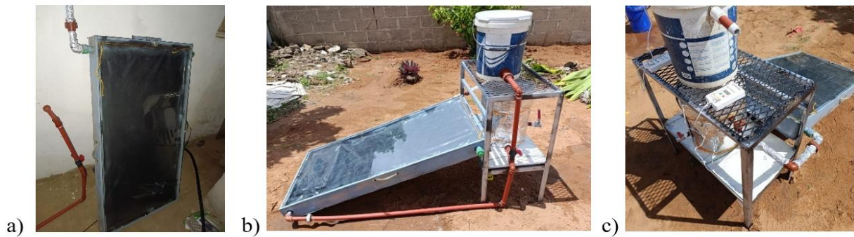
Legend: a) Alternative material collector plate; b) Alternative solar heater; c) Prototype under testing
