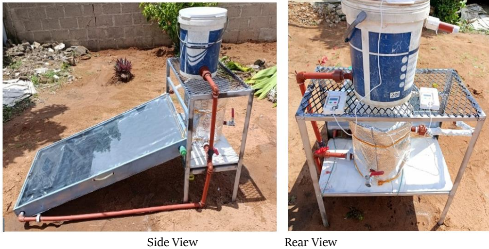
Figure 7: Solar Heater in Trials and Data Collection
